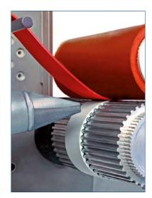
WHM offers a large spectrum of different coatings for rubber timing belts, polyure-thane timing belts as well as Vee-belts: Supergrip, Lnatex (also without butt-joint),
