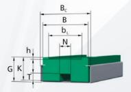
Version K, KC with V-guide (V-notch: 6 mm or 13 mm).
