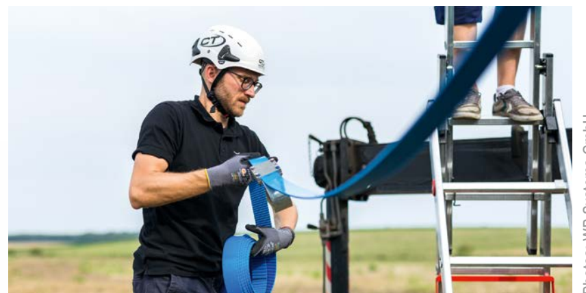
The 15.5 m long telescopic frame consists of several segments to permit transport on a trailer. It's a good thing that the timing belt of the same length is easy to roll up and unroll ...
