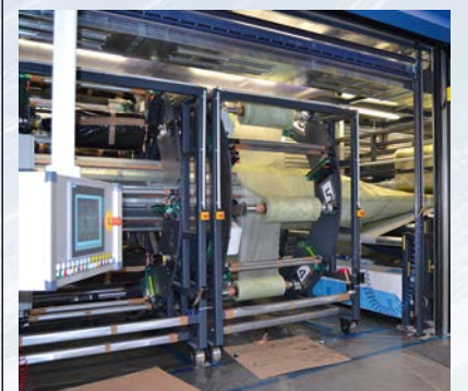
On a huge scale: A winding form measuring 4 m in width rotates around the tongue and winds the pre-impregnated glass fibre-reinforced webs around the tube film.
