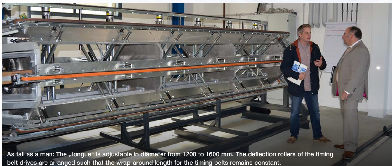
The 10 m long coated BRECOFLEX® BAT polyurethane timing belts help retain the shape of the film tube and transport them on to the winding station.
