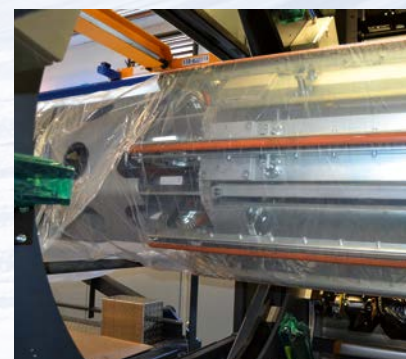
The 10 m long coated BRECOFLEX® BAT polyurethane timing belts help retain the shape of the film tube and transport them on to the winding station.
