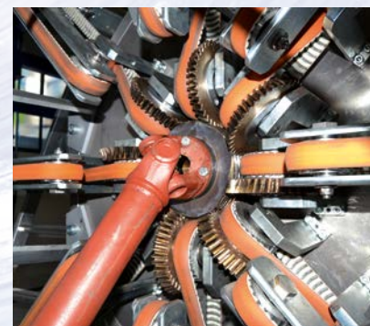
Mechanical work of art: The timing belts are driven via a drive shaft and a central worm gear at the front end of the tongue.
