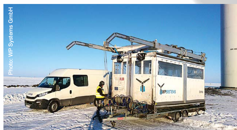
The tandem axis trailer with the service platform system terra 1.1 of WP Systems in Sweden. The permissible total weight of 3.5 tonnes must not be exceeded despite extensive system technology such as controls, power supply, cable winches, etc.
