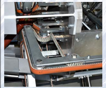
Adapted: the resistant linatrile backing is sanded according to the contour of the deflection rollers.
