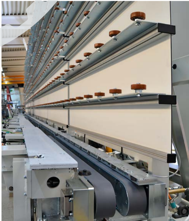
Timing belt drives in a row with the coated BRECOFLEX® AT515 for transport and precise positioning during CNC processing.
