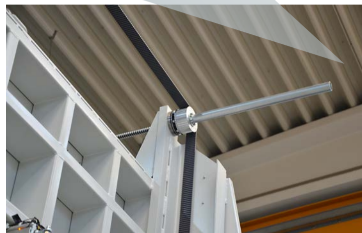
A clever solution: One joined BRECO® AT10 timing belt drives four spindle drives in the huge assembly and gas filling press.
