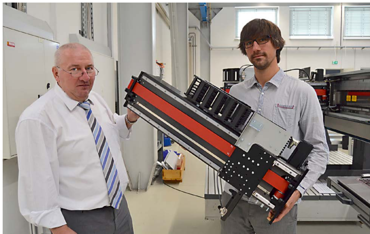
André Schmidt, customer consultant at Wilhelm Herm. Müller GmbH & Co. KG (on the left) and Bastian Sadewasser, design engineer at JAT. The innovative gantry made of CFRP is driven by a CONTI® SYNCHROFLEX GEN III timing belt and weighs only 5.2 kg.
