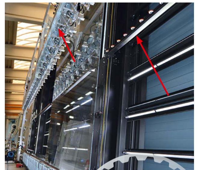
Inspection station: Dirt and scratches are made visible in front of the black background with special lighting. On the top left, the gripper beam; on the top right, the support beam with smaller rollers.
