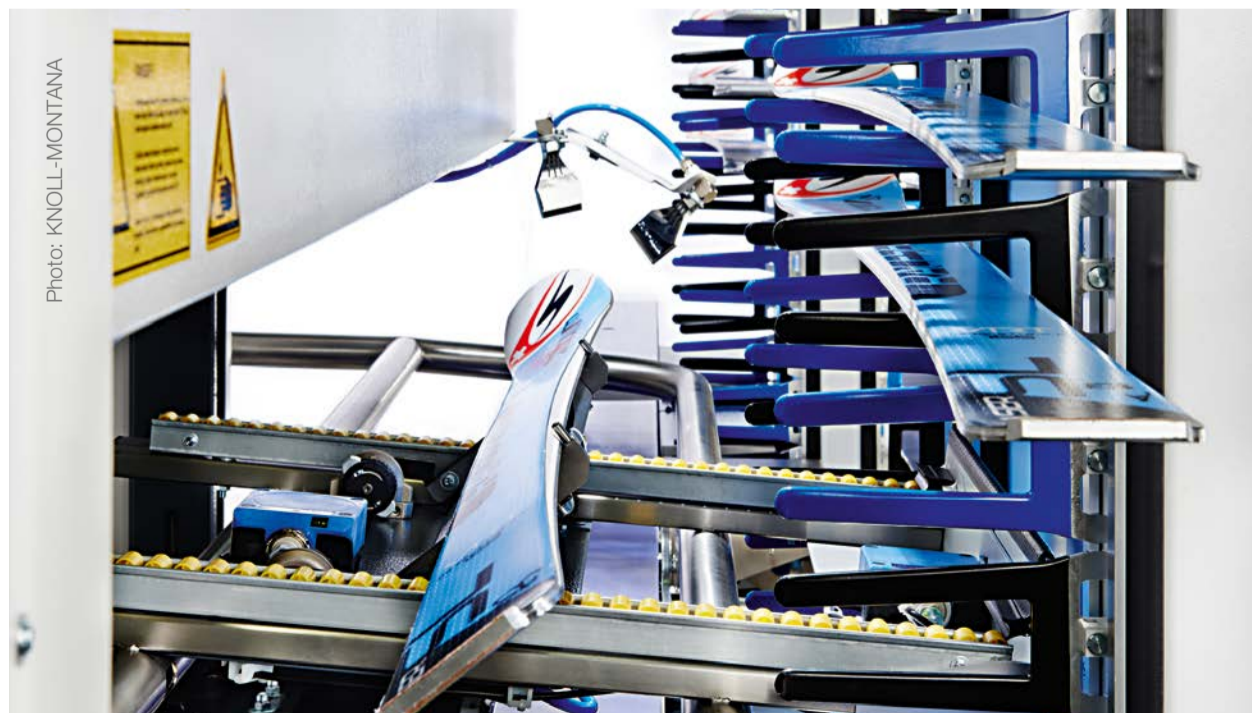
Transfer of the skis from the unloading level to the paternoster lift.
