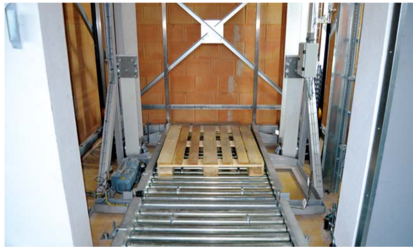
View from the roller conveyor to the lift cage and the two lateral timing belt drives.
