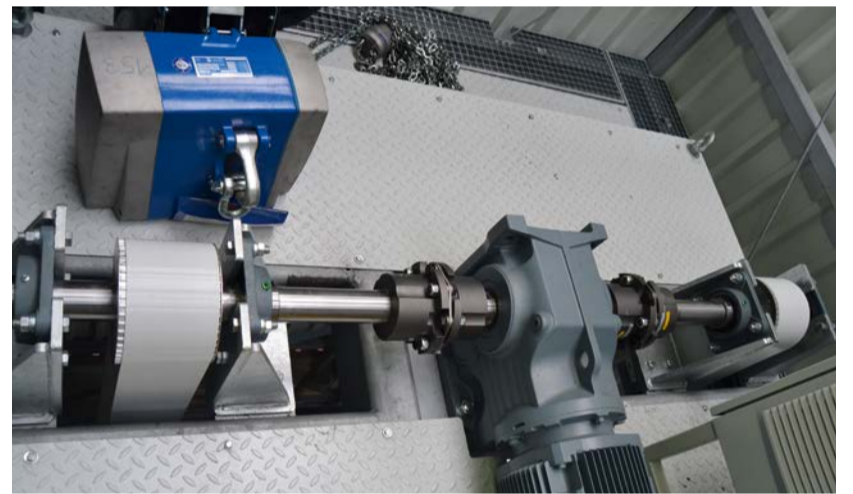
At the top: The geared servo motor distributes its torque via steel multiple-disc clutches to the pulleys.
