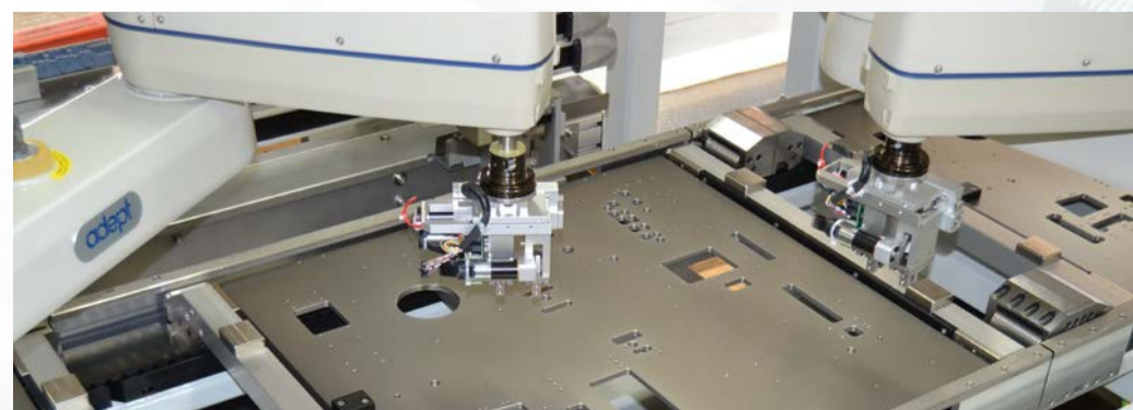
Robot station: The product carriers do not lie on the timing belt but on L-shaped stainless steel brackets that are fastened to belt cams and aluminium cross supports.
