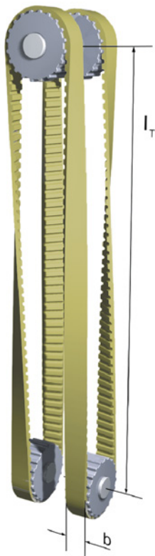
Angular drive with 2 axes
